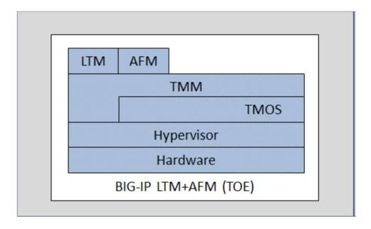
The TOE is separated into two (2) distinct planes, the control plane and the data plane. The control plane validates, stores, and passes configuration data to all necessary systems. It also provides all administrative access to the TOE. The data plane passes user traffic through the TOE.
